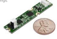
**How good is it?** Unlike standard sensors used in many towed arrays, SeaTRAX-85° delivers heading accuracies of 0.25° in the Arctic Circle - previously unheard of in a tiny digital magnetic compass module. Even at 85° latitude, it delivers better than 1.5° heading accuracy. So you get clear survey images even in the Arctic Ocean.
